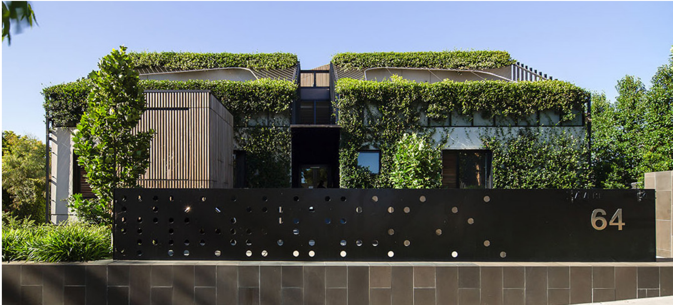
OPTION 2: Webnet Mesh with Trachelospermum jasminoides grown from roof and ground. Image supplied by JCB Architects. Project: Anderson Rd, Hawthorn East
